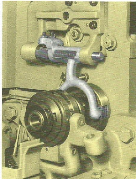
A disk brake added to the machine spindle is actuated between high and low speed.
