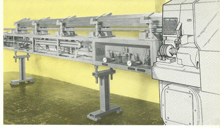
travel ejector pin, located within the Bar Feed Pusher, or by a momentary jet of air from the Air Eject Unit.
